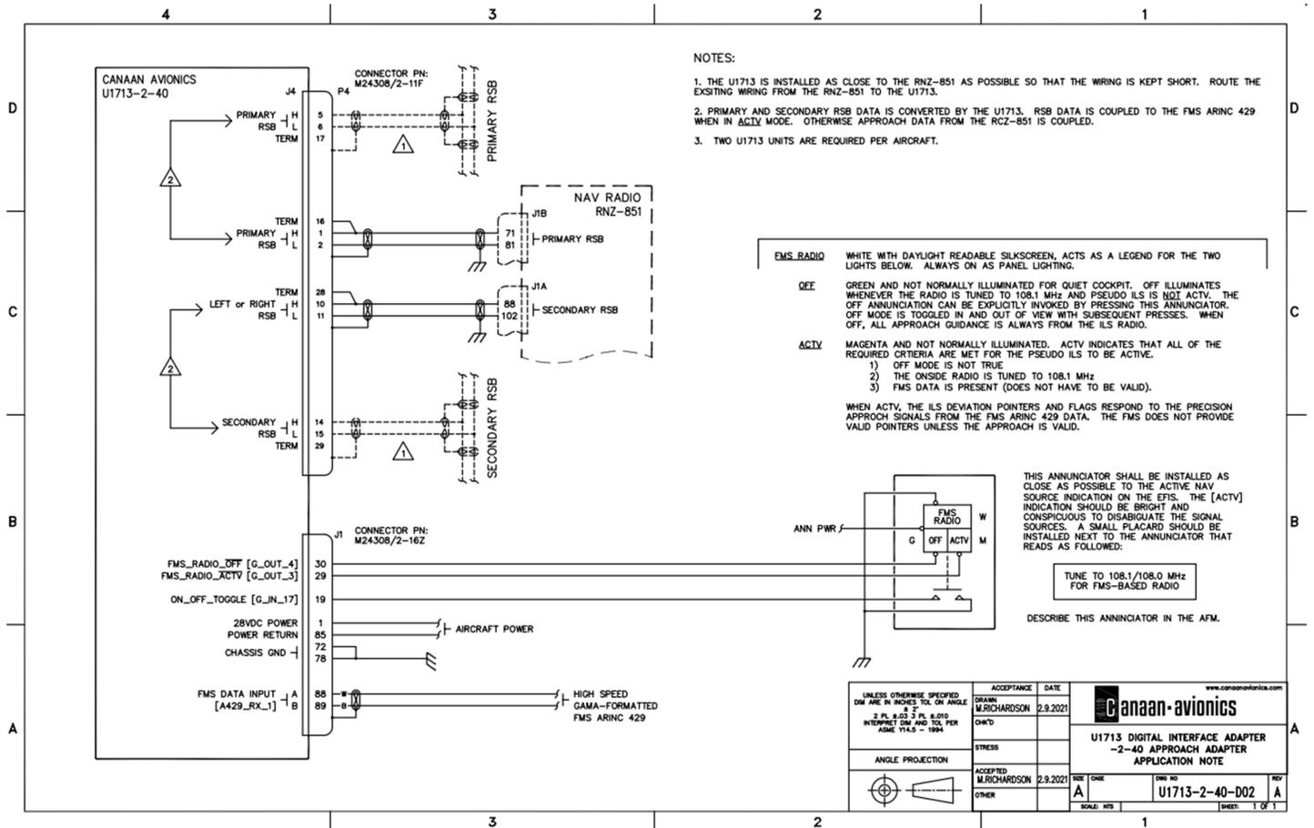
The example Application Note [above] is for the U1713-2-40 Approach Adapter. The Application Note identifies the ports used and how they are wired to other systems. The STC developer uses the Application Note [and this Installation Manual] to develop detailed Installation Drawings and to help develop Ground Test Plans and Flight Test Plans. Canaan Avionics uses the Application Note to communicate and validate the software functionality.
