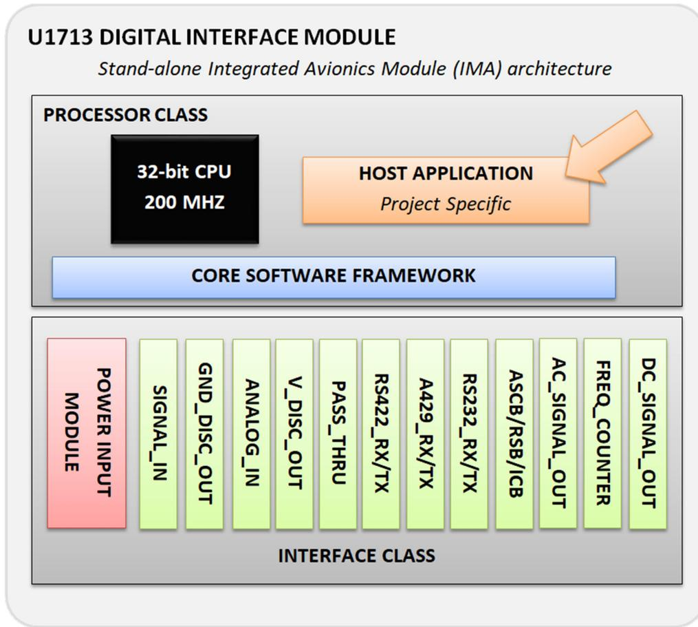
The unit has a single loadable software part that executes on a 200MHz ARM CPU. The U1713 contains no complex hardware as defined by AC 20-152, meaning that it is a simple processor/interface class module. Software on the device configures and has access to all of the ports available and drives all of the Signal Types.
